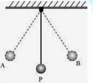
When an apparatus moves from its mean position P to either of its extreme positions A or B, it rises through a height h on top of the mean level P. At this time, the K.E. of the bob changes fully into P.E. The K.E. becomes zero, and also the bob possesses solely P.E. Because it moves towards purpose P, its P.E. decreases increasingly. Consequently, the
