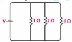
From the circuit, it is understood that all the resistors are connected in parallel. Therefore, their equivalent resistance can be calculated as follows:
