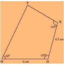
Draw a line segment MO of 6 cm and an angle of  $105^{\circ}$  at point O. As vertex R is 4.5 cm (1) away from the vertex O, cut a line segment OR of 4.5 cm from this ray.
