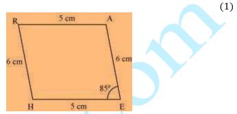
Draw a line segment HE of 5 cm and an angle of 85<sup>o</sup> at point E. As vertex A is 6 cm away from vertex E, cut a line segment EA of 6 cm from this ray.
