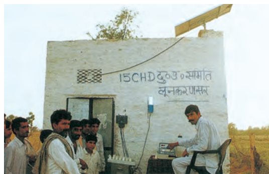
Fig. 5.11: Solar operated electronic milk testing equipment
